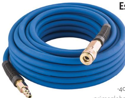
The Estwing E1450PVCR air hose is constructed of a flexible and durable hybrid blend of rubber and PVC. This 50-foot hose features corrosion-resistant, solid-brass fittings (1/4-inch NPT and universal coupler), bend resistors, a kink-resistant hose and all-weather flexibility from -40-164 degrees Fahrenheit.
